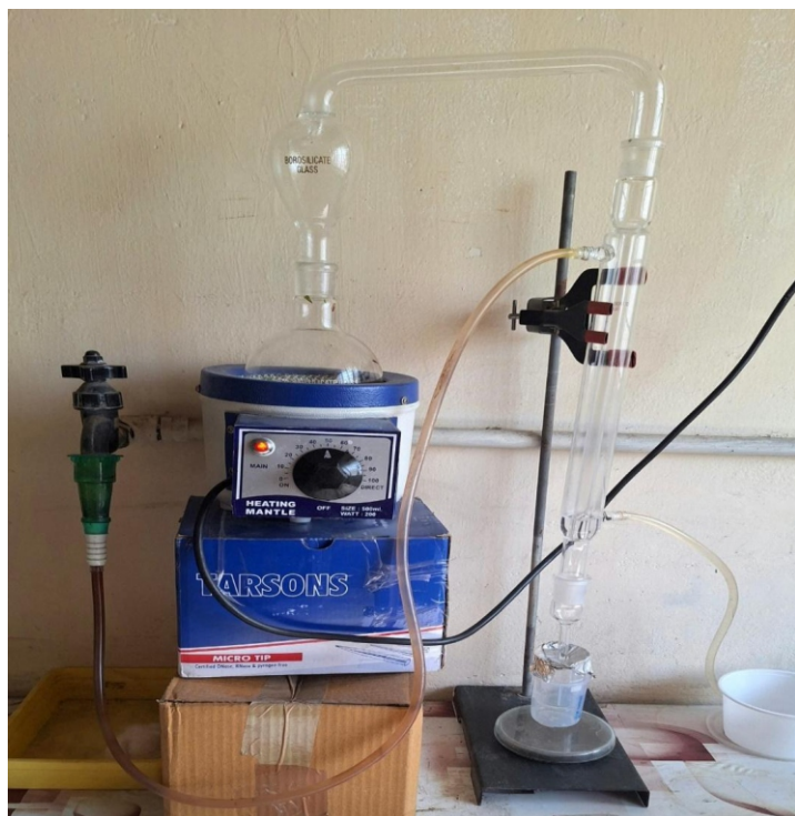
Figure 1: The above image depicts garlic oil extraction through steam distillation using a Soxhlet extractor
