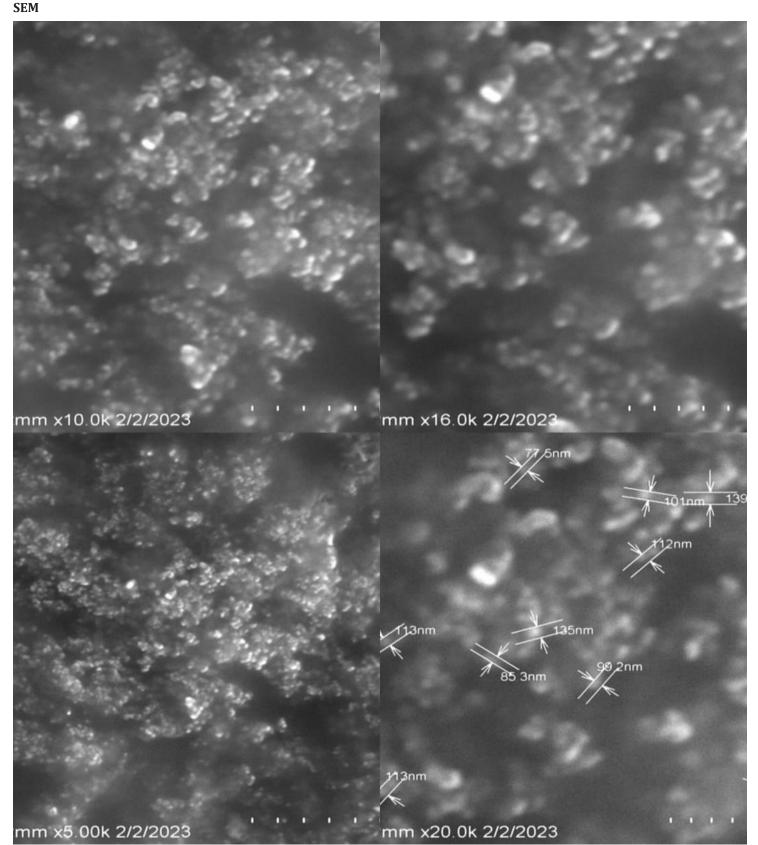
Scanning electron microscopy was used to research the formed and size characteristics of the created nanoparticles. A glass substrate was used to generate Zn nanoparticles in Figure employing ZnNPs collected from costus leaves. According to the results, ZnNPs were primarily homogenous in size, and their shape could be predicted. Most of the nanoparticles produced were spherical and ranged from 77 to 113 nm. The uniformly distributed Zn nanoparticles on the surface of the cells were observed.
